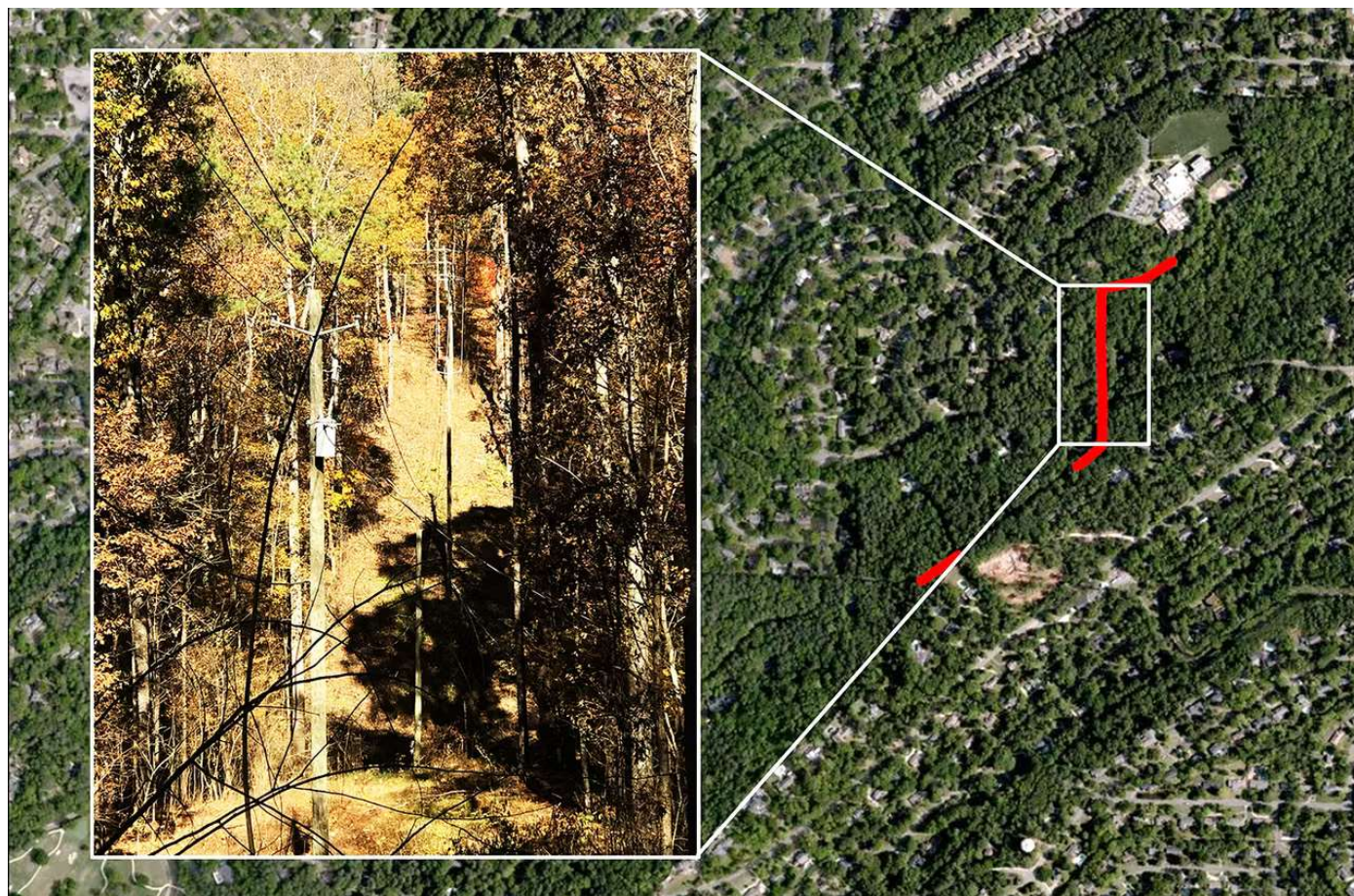
Fault Location halo on Mtn Site substation momentary event. View that evaluators and crews have in the field using Fault Location Reports which overlays the fault halo coordinates onto satellite images. Halos for momentary events are valuable since they can give clues where a fault will likely cause a sustained outage in the future—this one is in rear lot construction which is difficult to patrol, especially at night.
